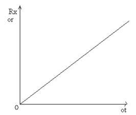
Transmitter Rotor Position Vs Receiver Rotor Position
