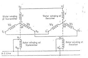
(a) Torque transmission using synchro transmitter.
